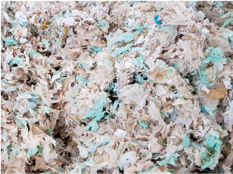
Figure 3 – AHP recycled plastic in sheets form Figure 4 – Separation system
